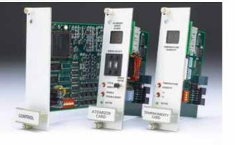
DURABLE, EASY TO MAINTAIN AND UPGRADE: UTILIZE SEVEN MONITORING/CONTROL CHANNELS AS EITHER SPEED CONTROL (MAXIMUM OF SIX) OR TEMPERATURE/HUMIDITY DISPLAYS (MAXIMUM OF FIVE). The Ransburg PulseTrack 2 is a microprocessor-based system designed to continuously monitor and maintain the programmable speeds of up to six rotary atomizers while also monitoring temperature and humidity for one or more zones.
