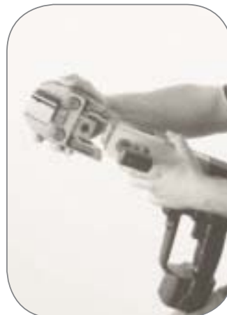
Place the jaws in the housing
